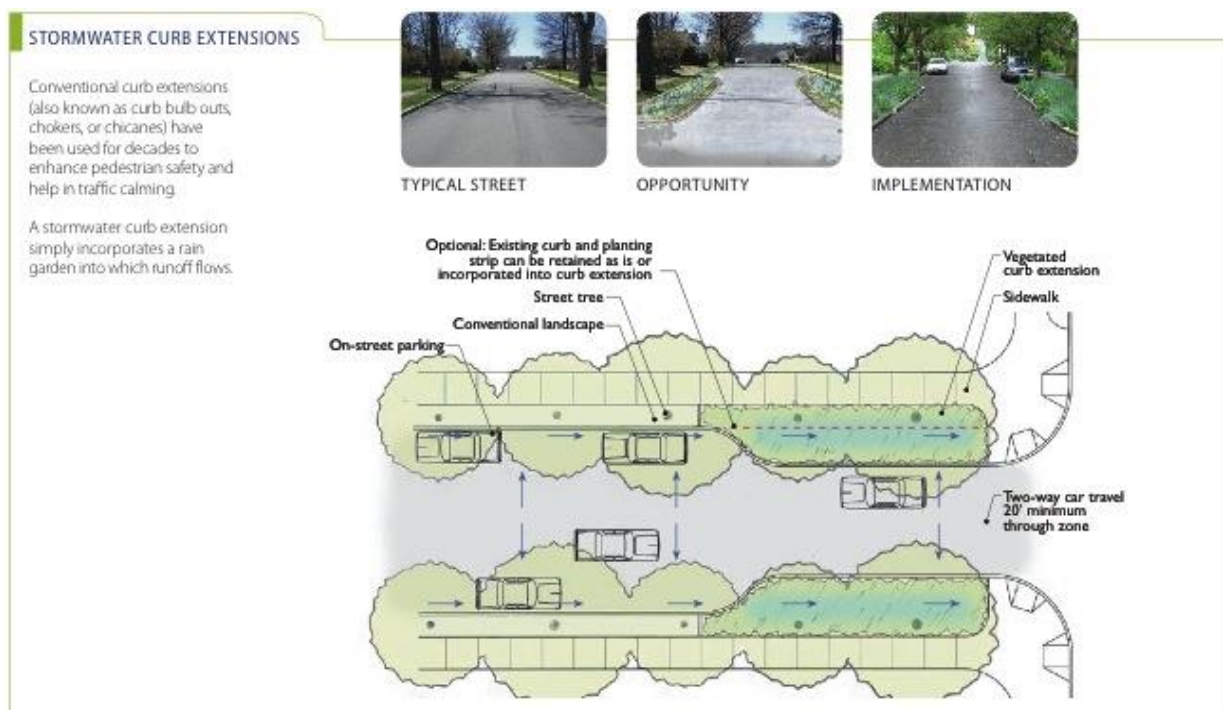
FIGURE 21: SCHEMATIC FOR STORMWATER CURB EXTENSIONS (EPA, 2009, GREEN STREETS)
