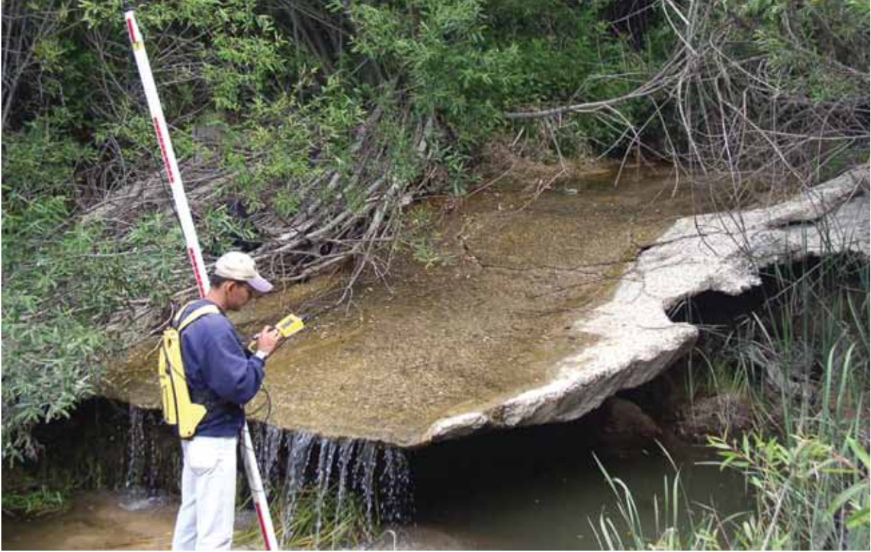
Stream Team staff mapping hardened streambank modification. Photo credit: Heal the Bay.
