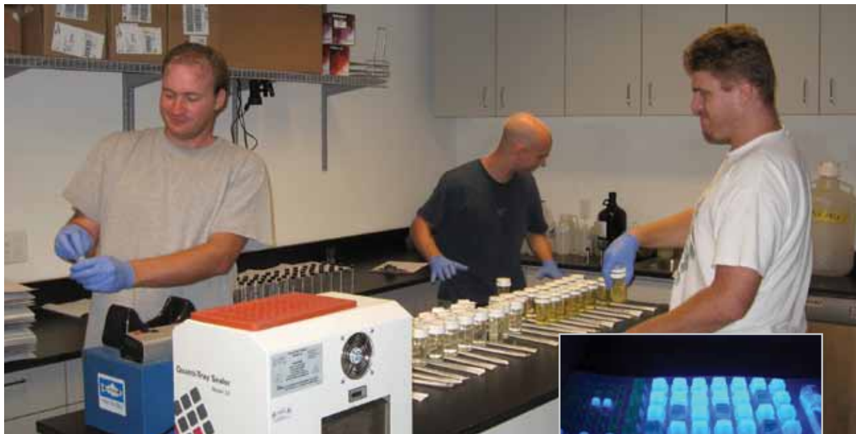
Stream Team staff and volunteers conduct laboratory testing for fecal indicator bacteria (top); a positive test for presence of fecal indicator bacteria (right).
