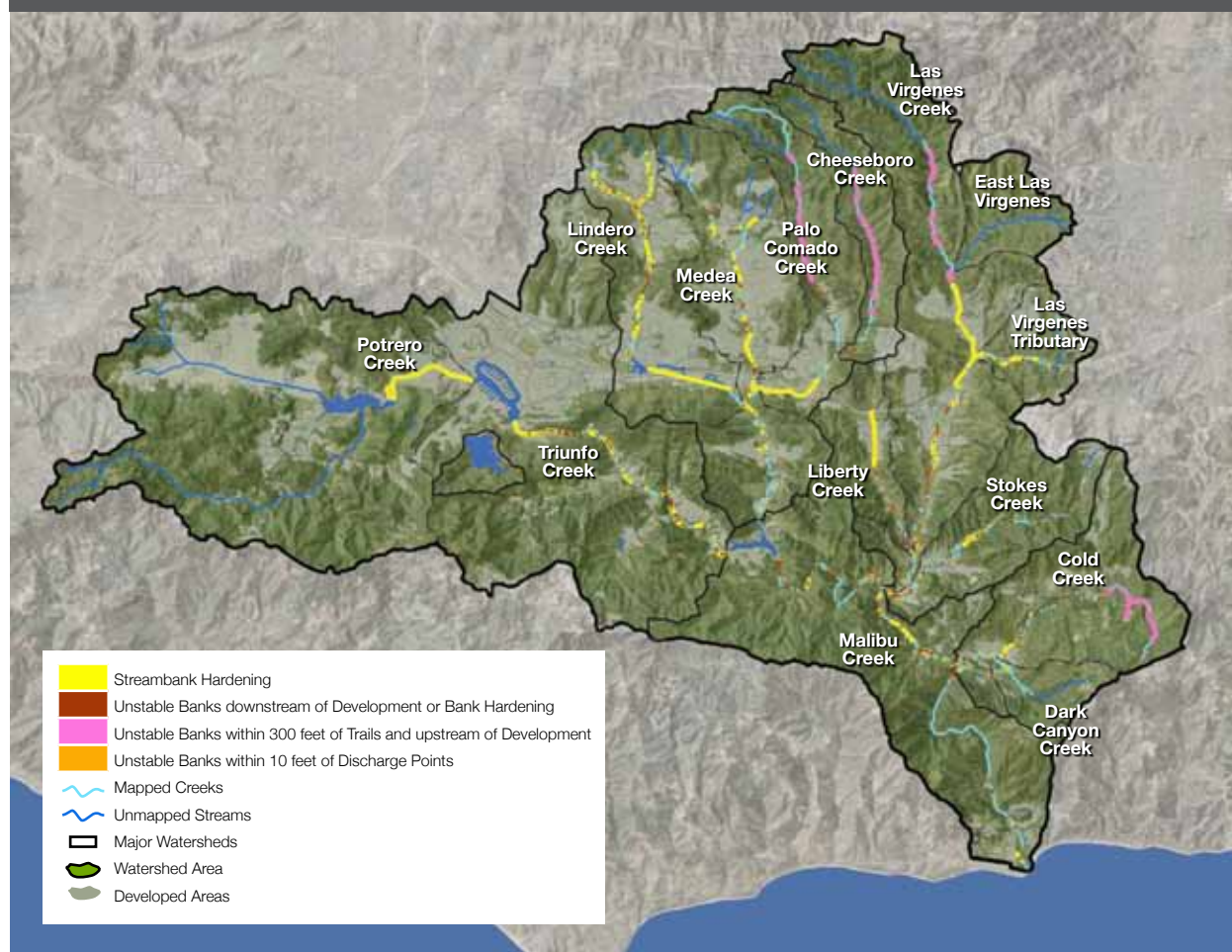
FIGURE 2-3: Streambank modifications and unstable streambanks throughout the Malibu Creek Watershed, mapped through Stream Walk (2000-2004).
