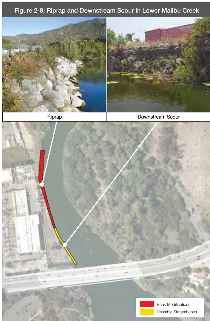
FIGURE 2-8: Digitized figure of riprap and downstream scour from 2000 to 2004 at the Mariposa property in lower Malibu Creek. Photos taken in 2011 to show similar conditions as previously mapped.
