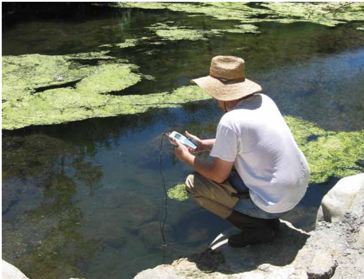
Stream Team staff measuring conductivity. Photo credit: Heal the Bay
